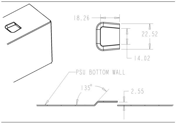
Figure 10. Power Supply Mounting Slot Detail
